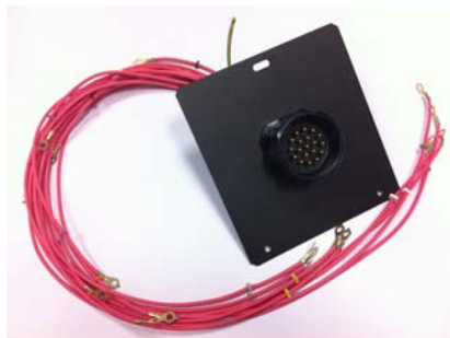
Internal adapters connecting sockets with new plate
