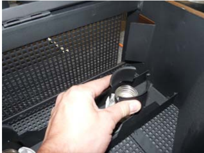
Press the support to facilitate the installation of reflectors
